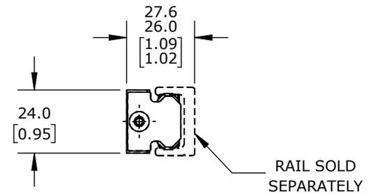
SINGLE ROW BALL BEARING, END SEAL, POLYACETAL/440C STAINLESS STEEL.
