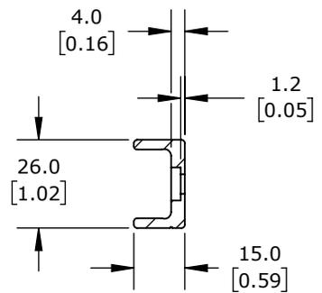
ANODIZED ALUMINUM, 15 X 26 X 1520mm. FOR USE WITH SUREMOTION LUC-1 SERIES CROWN CARRIAGES.
