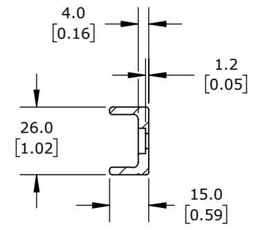
ANODIZED ALUMINUM, 15 X 26 X 1280mm. FOR USE WITH SUREMOTION LUC-1 SERIES CROWN CARRIAGES.
