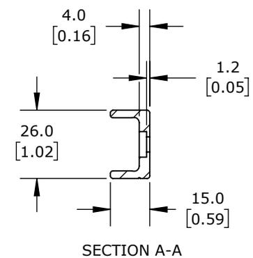
ANODIZED ALUMINUM, 15 X 26 X 1120mm. FOR USE WITH SUREMOTION LUC-1 SERIES CROWN CARRIAGES.
