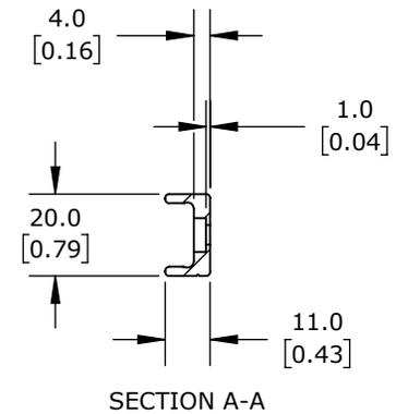
ANODIZED ALUMINUM, 11 X 20 X 960mm. FOR USE WITH SUREMOTION LUC-0 SERIES CROWN CARRIAGES.
