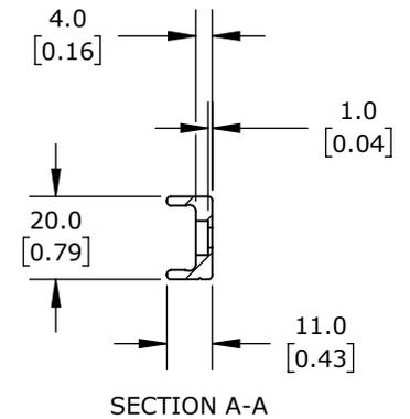
ANODIZED ALUMINUM, 11 X 20 X 800mm. FOR USE WITH SUREMOTION LUC-0 SERIES CROWN CARRIAGES.
