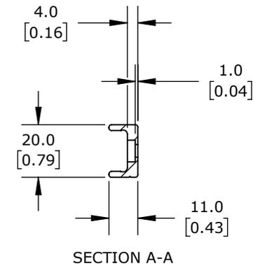
ANODIZED ALUMINUM, 11 X 20 X 640mm. FOR USE WITH SUREMOTION LUC-0 SERIES CROWN CARRIAGES.
