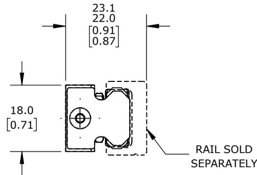
WHEN INSTALLING, ORIENT EMBOSSED ARROW IN THE DIRECTION OF THE APPLIED LOAD
