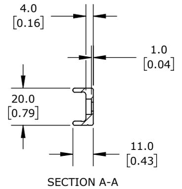
ANODIZED ALUMINUM, 11 X 20 X 480mm. FOR USE WITH SUREMOTION LUC-0 SERIES CROWN CARRIAGES.
