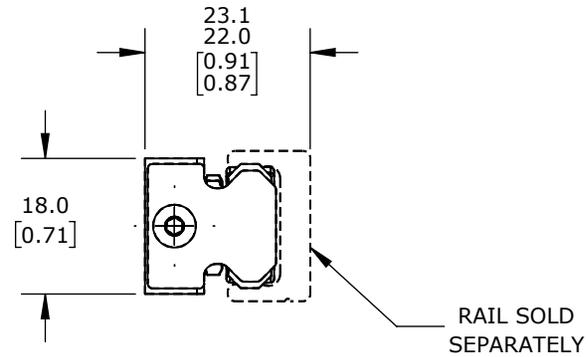
SINGLE ROW BALL BEARING, END SEAL, POLYACETAL/440C STAINLESS STEEL.
