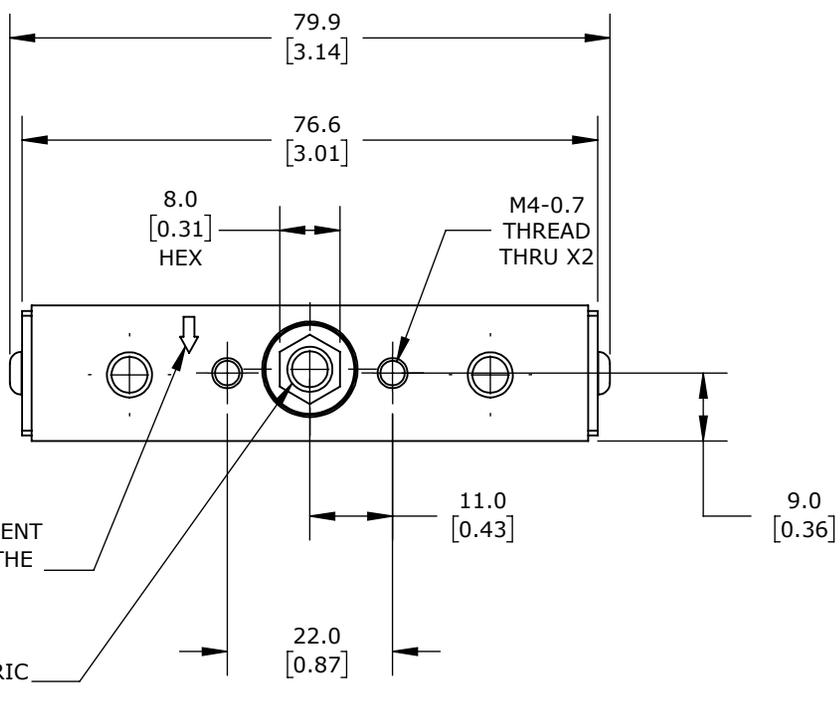
WHEN INSTALLING, ORIENT EMBOSSED ARROW IN THE DIRECTION OF THE APPLIED LOAD
