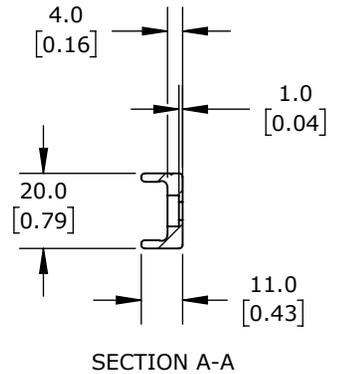
ANODIZED ALUMINUM, 11 X 20 X 1520mm. FOR USE WITH SUREMOTION LUC-0 SERIES CROWN CARRIAGES.
