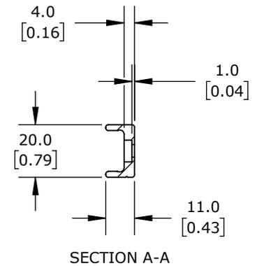
ANODIZED ALUMINUM, 11 X 20 X 1120mm. FOR USE WITH SUREMOTION LUC-0 SERIES CROWN CARRIAGES.
