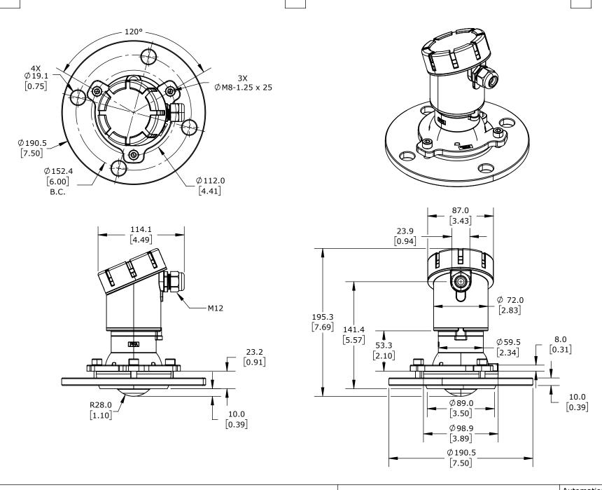
FLOWLINE GP RADAR LEVEL SENSOR
