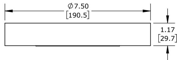
FLOWLINE MOUNTING FLANGE, CPVC, 3IN ANSI X 1-1/2IN FEMALE NPT, FOR USE WITH FLOWLINE ECHOBEAM
