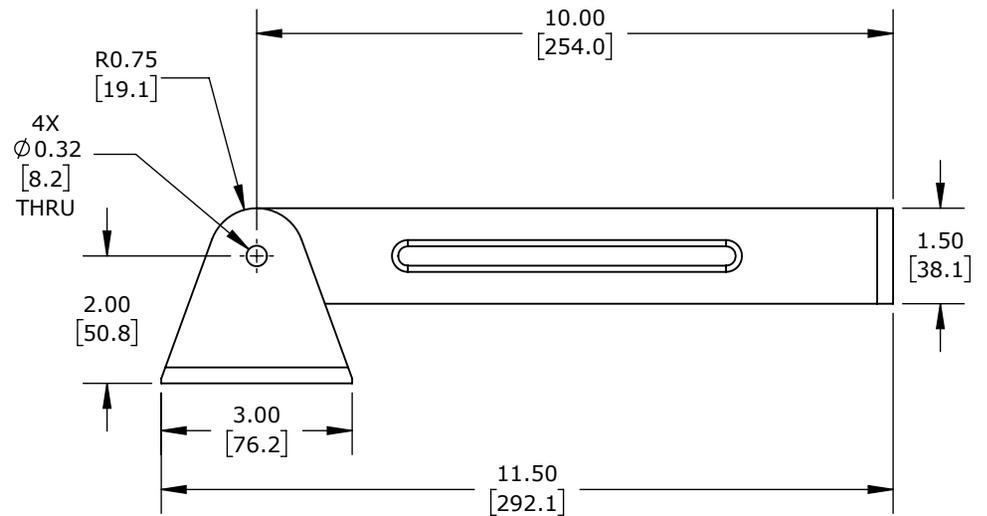
FLOWLINE LONG MOUNTING BRACKET, 316 STAINLESS STEEL. FOR USE WITH FLOWLINE ECHOBEAM FREQUENCY MODULATED CONTINUOUS WAVE (FMCW) RADAR LEVEL SENSORS. 1-1/2IN NPT LOCK NUT INCLUDED.
