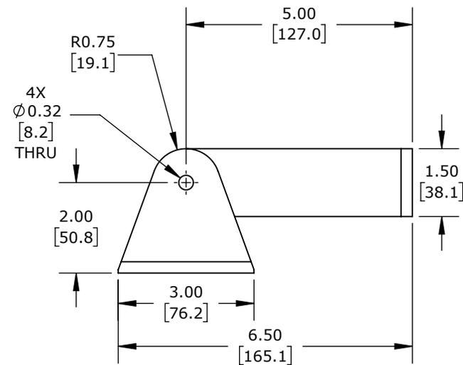
FLOWLINE SHORT MOUNTING BRACKET, 316 STAINLESS STEEL. FOR USE WITH FLOWLINE ECHOBEM FREQUENCY MODULATED CONTINUOUS WAVE (FMCW) RADAR LEVEL SENSORS. 1-1/2IN NPT LOCK NUT INCLUDED.
