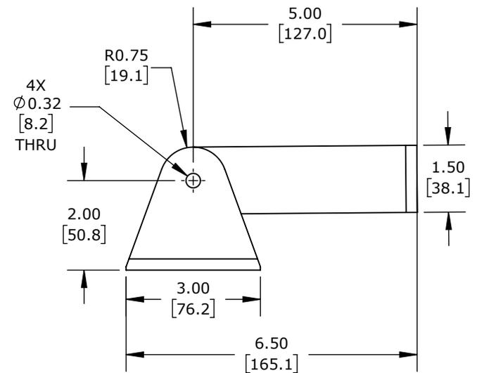
FLOWLINE SHORT MOUNTING BRACKET, 316 STAINLESS STEEL. FOR USE WITH FLOWLINE ECHOBEM FREQUENCY MODULATED CONTINUOUS WAVE (FMCW) RADAR LEVEL SENSORS. 1IN NPT LOCK NUT INCLUDED.
