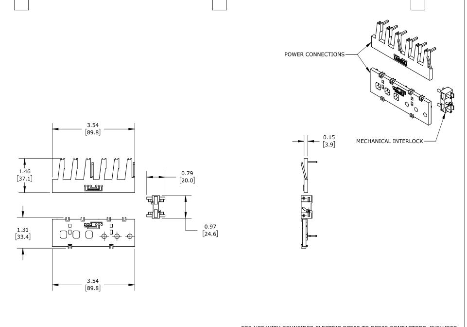
FOR USE WITH SCHNEIDER ELECTRIC DPE09 TO DPE38 CONTACTORS, INCLUDES LINE AND LOADSIDE CONNECTION BARS AND MECHANICAL INTERLOCK.
