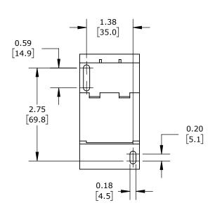
FOR USE WITH SCHNEIDER ELECTRIC DPER01 TO DPER32 THERMAL OVERLOAD RELAYS.
