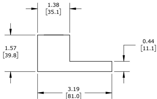
BOX TYPE, ALUMINUM-TIN PLATED, 600V, 1 OPENINGS, (1) 2 AWG-600 MCM COPPER OR (1) 2 AWG-600 MCM ALUMINUM, AL9CU.
