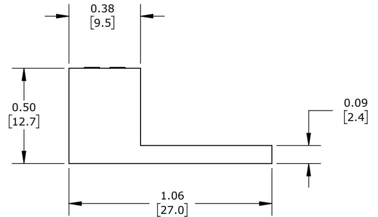
BOX TYPE, ALUMINUM-TIN PLATED, 600V, 1 OPENINGS, (1) 14-4 AWG COPPER OR (1) 8-4 AWG ALUMINUM, AL9CU.
