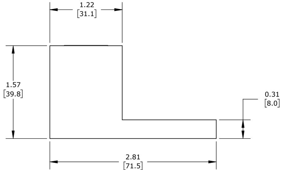
BOX TYPE, ALUMINUM-TIN PLATED, 600V, 1 OPENINGS, (1) 4 AWG-500 MCM COPPER OR (1) 4 AWG-500 MCM ALUMINUM, AL9CU.
