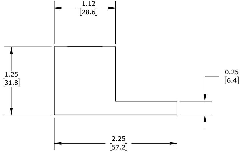
BOX TYPE, ALUMINUM-TIN PLATED, 600V, 1 OPENINGS, (1) 6 AWG-350 MCM COPPER OR (1) 6 AWG-350 MCM ALUMINUM, AL9CU.
