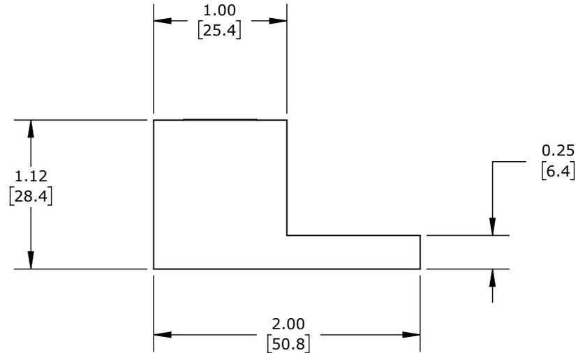
BOX TYPE, ALUMINUM-TIN PLATED, 600V, 1 OPENINGS, (1) 6 AWG-250 MCM COPPER OR (1) 6 AWG-250 MCM ALUMINUM, AL9CU.
