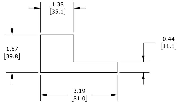
BOX TYPE, ALUMINUM-TIN PLATED, 600V, 2 OPENINGS, (1) 2 AWG-600 MCM COPPER OR (1) 2 AWG-600 MCM ALUMINUM, AL9CU.
