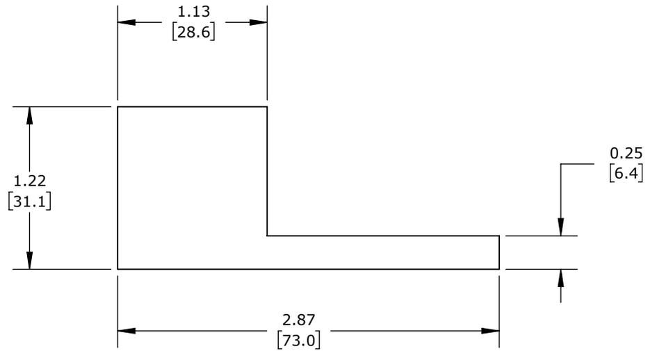
BOX TYPE, ALUMINUM-TIN PLATED, 600V, 2 OPENINGS, (1) 6 AWG-350 MCM COPPER OR (1) 6 AWG-350 MCM ALUMINUM, AL9CU.
