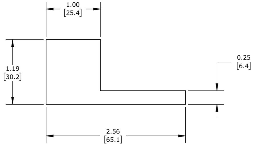
BOX TYPE, ALUMINUM-TIN PLATED, 600V, 2 OPENINGS, (1) 6 AWG-250 MCM COPPER OR (1) 6 AWG-250 MCM ALUMINUM, AL9CU.
