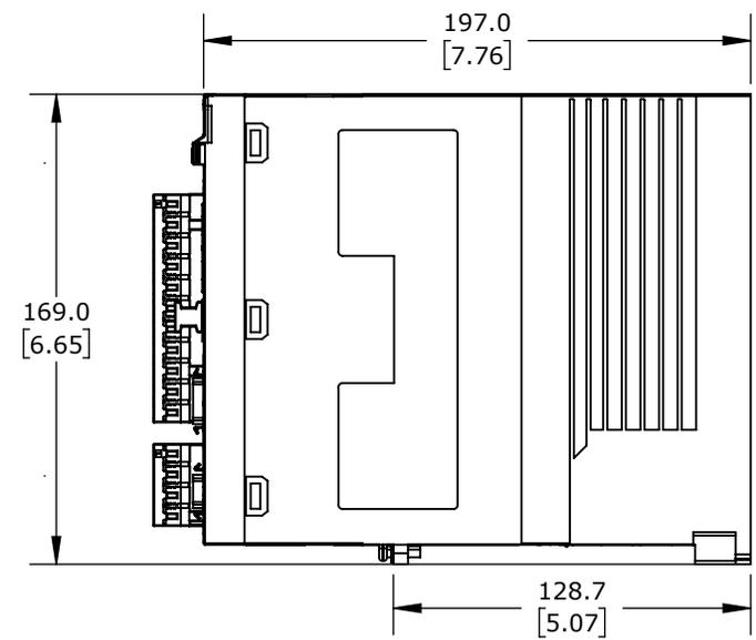
LS ELECTRIC SERVO DRIVE, 750W, 110/230 VAC 1 and 3-PHASE, (2) ETHERNET 100Base-TX (RJ45) PORT(S), EtherCAT and MODBUS TCP, FOR USE WITH 750W SYSTEMS
