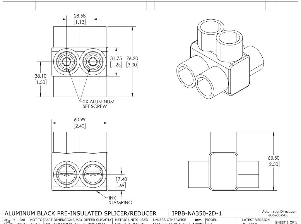
ANGLE | SCALE | DUE TO MANUFACTURER'S VARIANCES SPECIFIED UNITS ARE: [inch] REV. FOR PART DESIGN 9/2/2025
