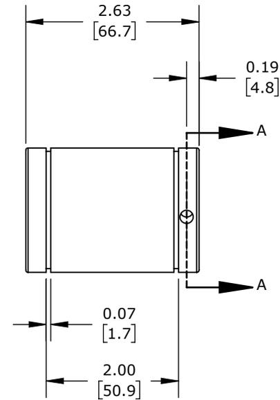
**PBC IP OPEN FULL BALL RECIRCULATING BEARING**
