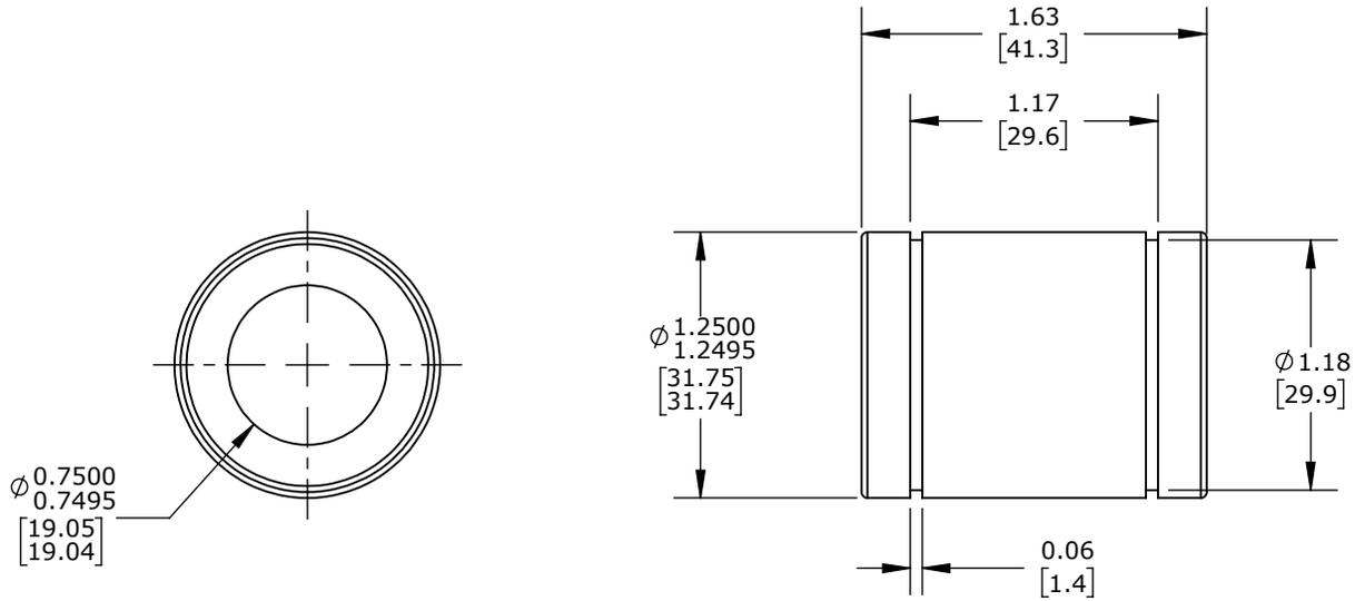
**PBC IP CLOSED FULL BALL RECIRCULATING BEARING**
