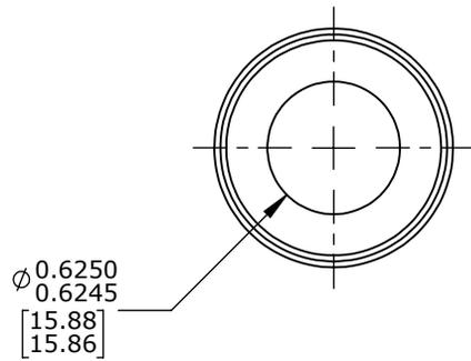
**PBC IP CLOSED FULL BALL RECIRCULATING BEARING**
