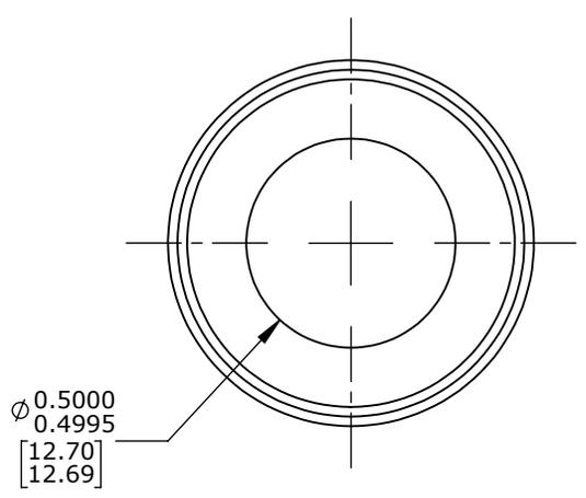
**PBC IP CLOSED FULL BALL RECIRCULATING BEARING**
