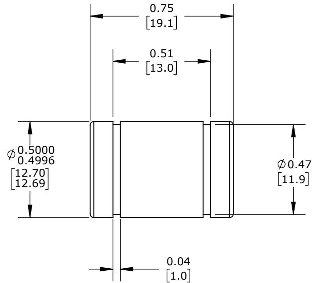
PBC IP CLOSED FULL BALL RECIRCULATING BEARING
