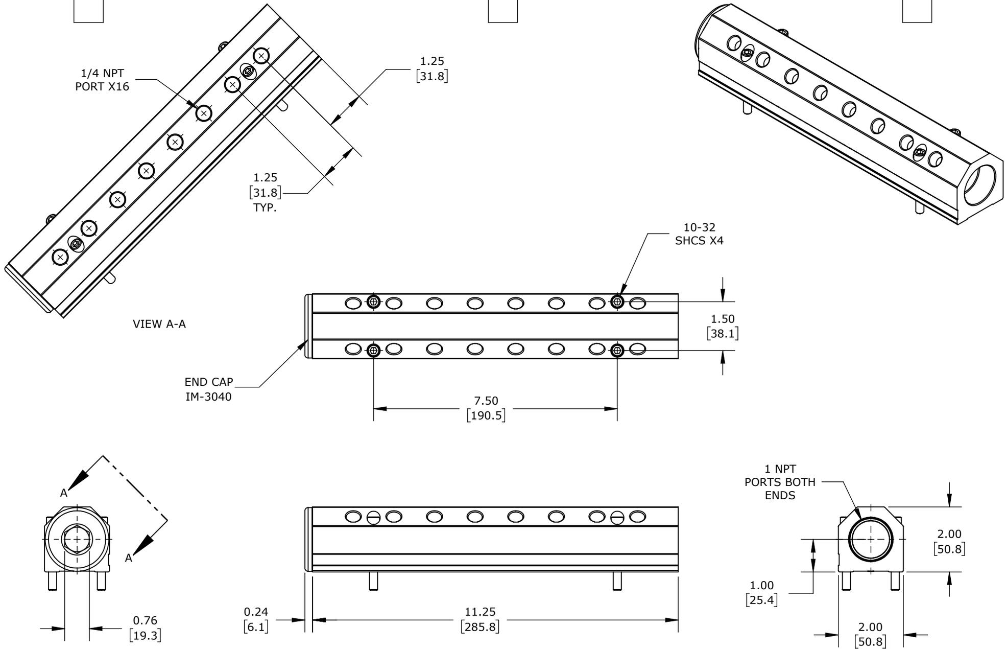
BLUE ANODIZED ALUMINUM, RECTANGULAR, 3000 PSI MAXIMUM OPERATING PRESSURE, (8) STATIONS, 1IN FEMALE NPT INLET(s), 1/4IN FEMALE NPT OUTLET(s), 45-DEG AND 135-DEG ORIENTATION.
