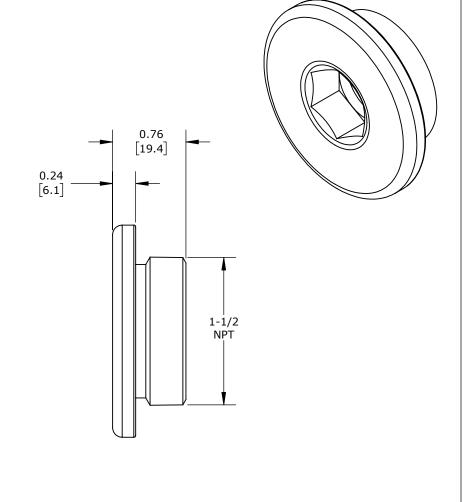
1-1/2IN MALE NPT, ANODIZED ALUMINUM. O-RING INCLUDED O-RING P/N IS #226
