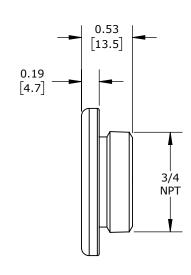
$3/4 \mbox{IN}$  MALE NPT, ANODIZED ALUMINUM. O-RING INCLUDED. O-RING P/N IS #123
