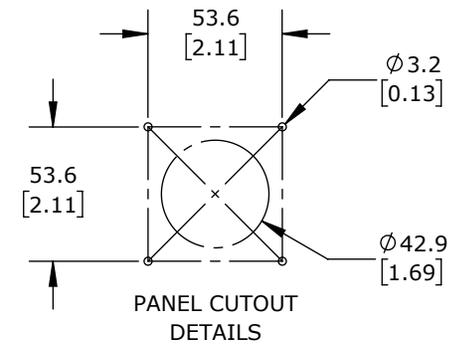
SELECTOR, BLACK, EXTERNAL FRONT MOUNT, 2-POSITION, LOCKABLE IN ON-OFF, DEFEATABLE, NEMA 3R, IP65. FOR USE WITH HMMP-63H MANUAL MOTOR PROTECTORS. 315mm SHAFT, OPERATOR AND MOUNTING SCREWS INCLUDED.
