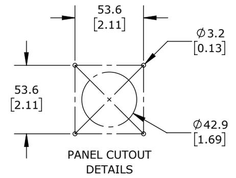
SELECTOR, BLACK, EXTERNAL FRONT MOUNT, 2-POSITION, LOCKABLE IN ON-OFF, DEFEATABLE, NEMA 3R, IP65. FOR USE WITH HMMP-63H MANUAL MOTOR PROTECTORS. 115mm SHAFT, OPERATOR AND MOUNTING SCREWS INCLUDED.
