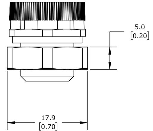
M12 X 1.5MM THREAD TYPE, POLYAMIDE, BLACK, 2000 ML/MIN @ 70 mbar (1 PSI), IP66 IP68, UL TYPE 4X. PACKAGE OF 2.
