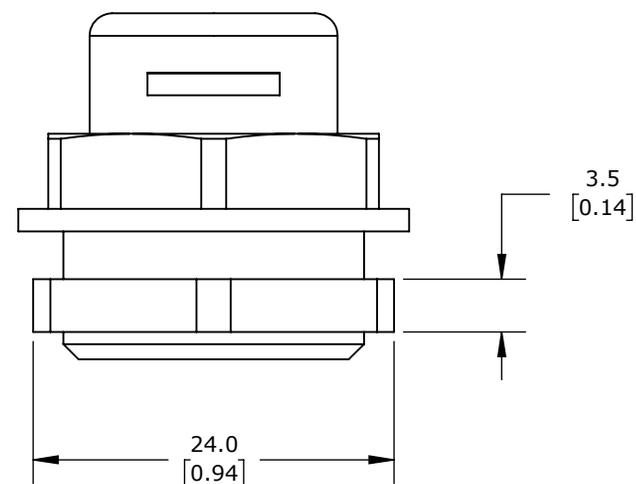
M20 X 1.5MM THREAD TYPE, STAINLESS STEEL, 2000 ML/MIN @ 70 mbar (1 PSI), IP66 IP68. PACKAGE OF 1.
