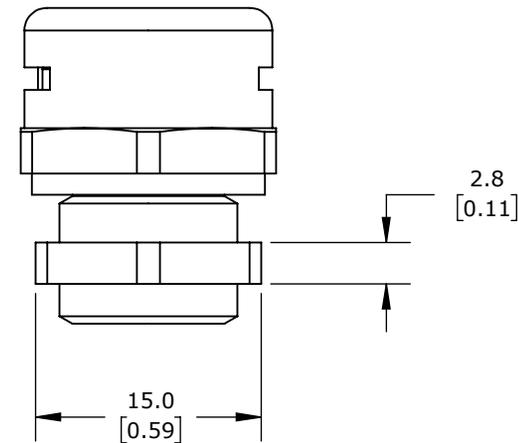
M12 X 1.5MM THREAD TYPE, STAINLESS STEEL, 2000 ML/MIN @ 70 mbar (1 PSI), IP66 IP68, UL TYPE 4X. PACKAGE OF 1.
