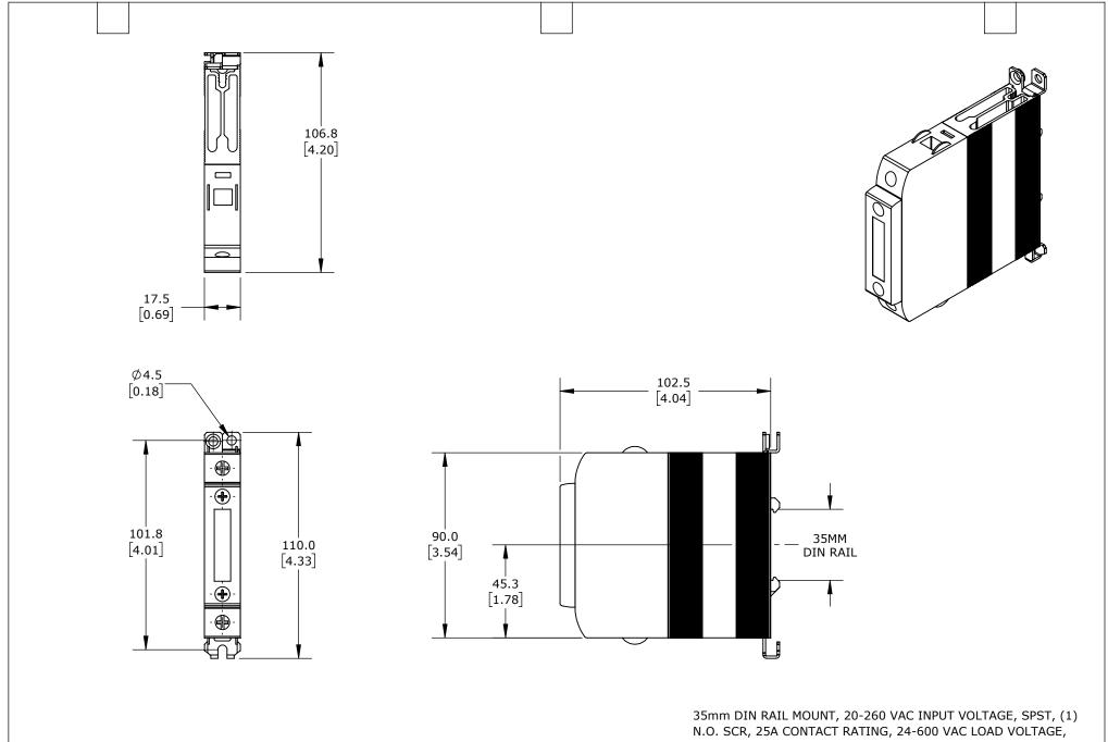
N.O. SCR, 25A CONTACT RATING, 24-600 VAC LOAD VOLTAGE,
