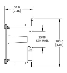
FINGER-SAFE, 510A, 1-POLE, LINE SIDE: 2 OPENINGS ACCEPT 250 KCMIL TO 4 AWG, LOAD SIDE: 2 OPENINGS ACCEPT 250 KCMIL TO 4 AWG, DIN RAIL OR PANEL MOUNT, UL 1059 RECOGNIZED.
