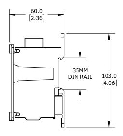
FINGER-SAFE, 420A, 1-POLE, LINE SIDE: 1 OPENING ACCEPTS FLAT BUSBAR, LOAD SIDE: 2 OPENINGS ACCEPT 2 AWG TO 14 AWG & 5 OPENINGS ACCEPT 6 AWG TO 14 AWG & 4 OPENINGS ACCEPT 8 AWG TO 14 AWG, DIN RAIL OR PANEL MOUNT, UL 1059 RECOGNIZED.
