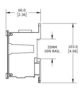
FINGER-SAFE, 400A, 1-POLE, LINE SIDE: 2 OPENINGS ACCEPT 250 KCMIL TO 4 AWG, LOAD SIDE: 12 OPENINGS ACCEPT 6 AWG TO 14 AWG, DIN RAIL OR PANEL MOUNT, UL 1059 RECOGNIZED.
