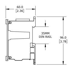
FINGER-SAFE, 335A, 1-POLE, LINE SIDE: 1 OPENING ACCEPTS 400 KCMIL TO 3/0 AWG, LOAD SIDE: 2 OPENINGS ACCEPT 2 AWG TO 14 AWG & 5 OPENINGS ACCEPT 6 AWG TO 14 AWG & 4 OPENINGS ACCEPT 8 AWG TO 14 AWG, DIN RAIL OR PANEL MOUNT.
