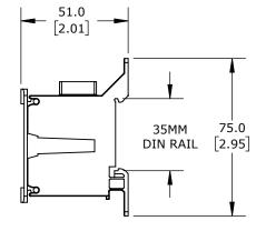
FINGER-SAFE, 250A, 1-POLE, LINE SIDE: 1 OPENING ACCEPTS FLAT BUSBAR, LOAD SIDE: 6 OPENINGS ACCEPT 6 AWG TO 14 AWG, DIN RAIL OR PANEL MOUNT, UL 1059 RECOGNIZED.
