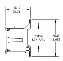
FINGER-SAFE, 175A, 3-POLE, LINE SIDE: 1 OPENING ACCEPTS 2/0 AWG TO 6 AWG, LOAD SIDE: 1 OPENING ACCEPTS 6 AWG TO 10 AWG & 6 OPENINGS ACCEPT 6 AWG TO 14 AWG, DIN RAIL OR PANEL MOUNT, UL 1059 RECOGNIZED.
