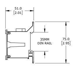
FINGER-SAFE, 160A, 1-POLE, LINE SIDE: 1 OPENING ACCEPTS 2/0 AWG TO 6 AWG, LOAD SIDE: 1 OPENING ACCEPTS 6 AWG TO 10 AWG & 6 OPENINGS ACCEPT 6 AWG TO 14 AWG, DIN RAIL OR PANEL MOUNT, UL 1059 RECOGNIZED.
